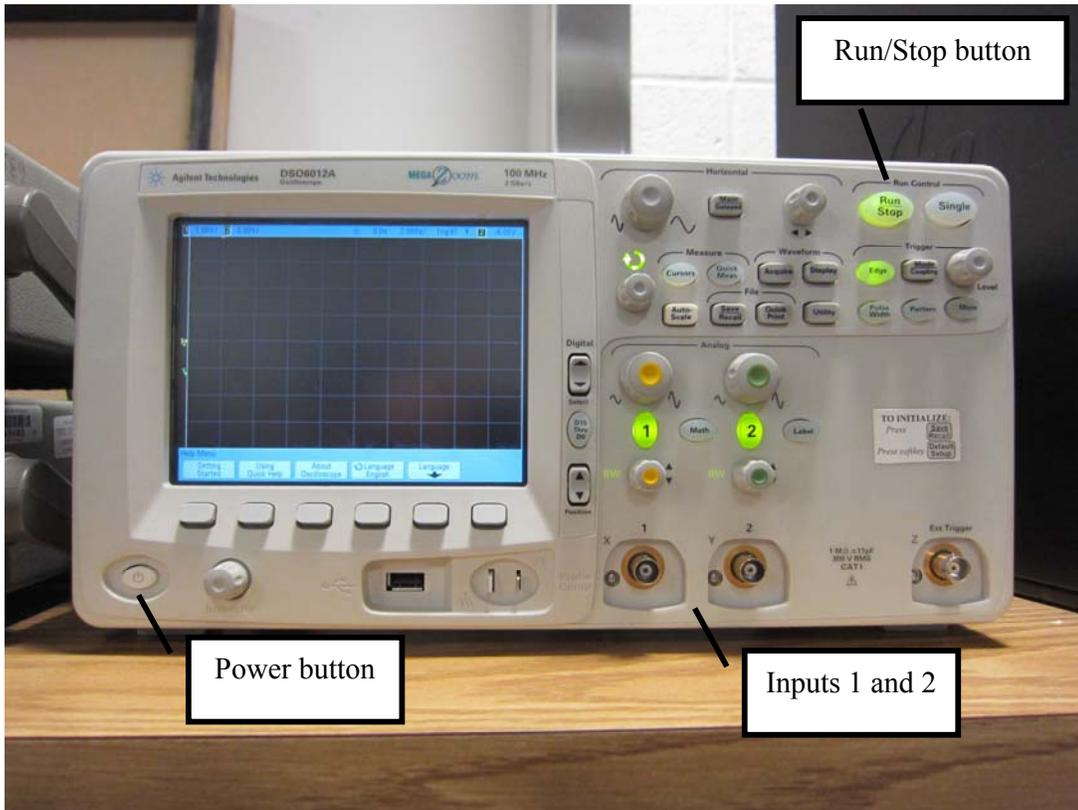
Figure 2 - Oscilloscope
