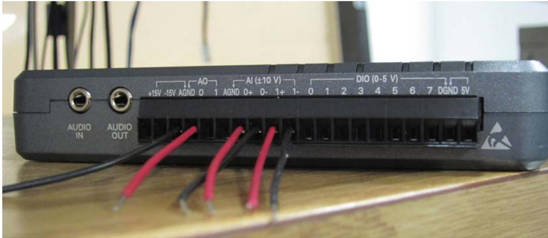
Figure 4 - Input/Output Connector on the myRIO
