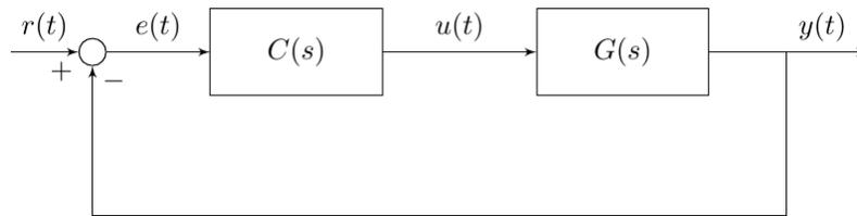
Figure 2-Closed Loop System
