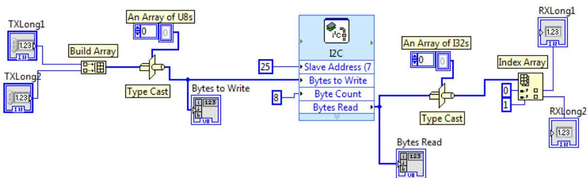
The "Type Cast" block and arrays are a bit confusing at first in LabView. Our goal for our code is to take 4 I16 Control variables and convert them to their 2 byte elements and send an 8 byte array of U8s to the I2C block. Then the I2C block will send those 8 U8s to the MSP430 and then read 8 more U8s from the MSP430. Then we need to take those 8 U8s in Labview and put them into I16 variables. The Type Cast
