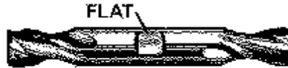
FIGURE1--The flat area on a commercial double-ended end mill is for the set screw on the end mill holder to tighten against.
