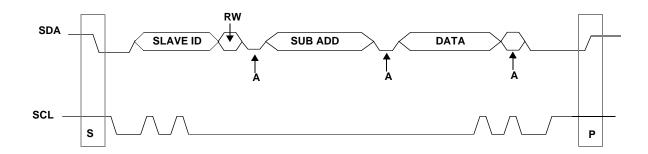
Figure 10. Data Transfer on the I<sup>2</sup>C Bus
