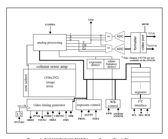
Figure 1. OV6620/OV6120 CMOS Image Sensor Block Diagram
