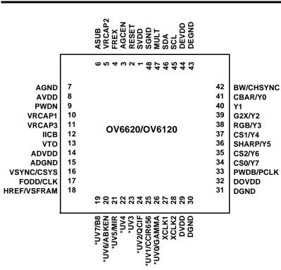
\* Note: Outputs UV0-UV7 are not available on the OV6120. The inputs associated with these respective pins are still functional.
