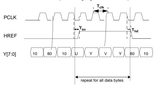
Pixel Data 8-bit Timing (PCLK rising edge latches data bus)
