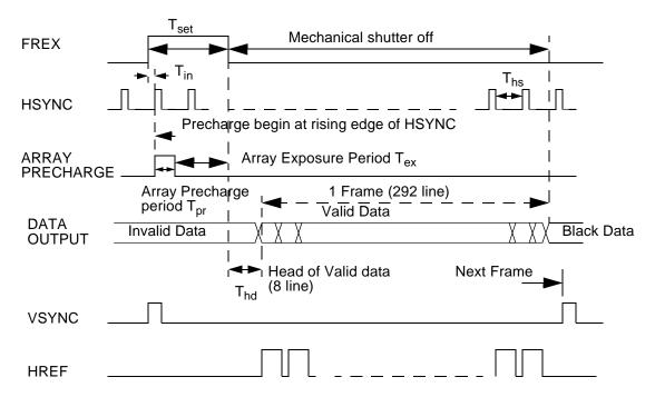
Note:  $T_{pr} = 292^* 4 * T_{clk}$ ,  $T_{clk}$  is internal pixel period. For default 17.73 MHz,  $T_{clk} = 112$  us. If CLK[5:0] set to divided number,  $T_{clk}$  will increase accordingly.
