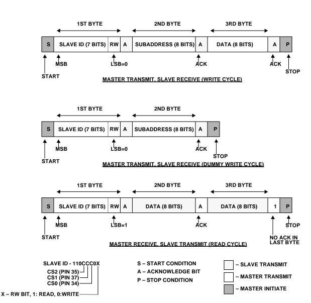
Figure 8. I<sup>2</sup>C Bus Protocol Format
