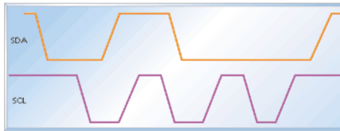
A start condition, a one data, a zero data bit, and a stop condition
