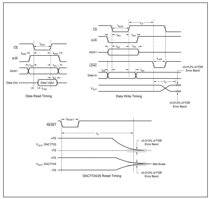
FIGURE 4. Digital Input and Output Timing.
