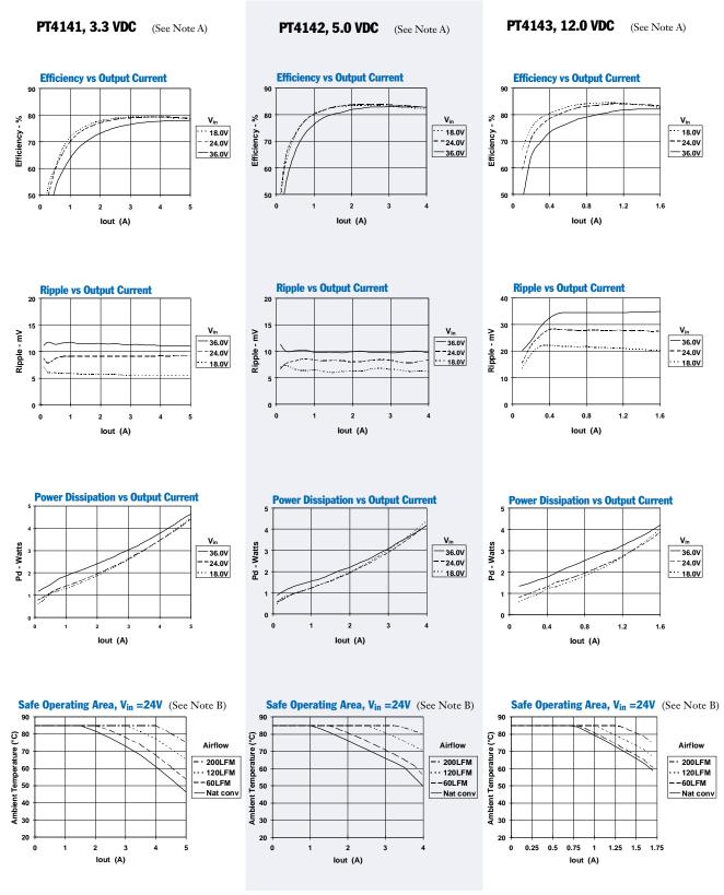
**Note A:** Characteristic data has been developed from actual products tested at 25°C. This data is considered typical data for the Converter. **Note B:** SOA curves represent the conditions at which internal components are at or below the manufacturer's maximum operating temperatures
